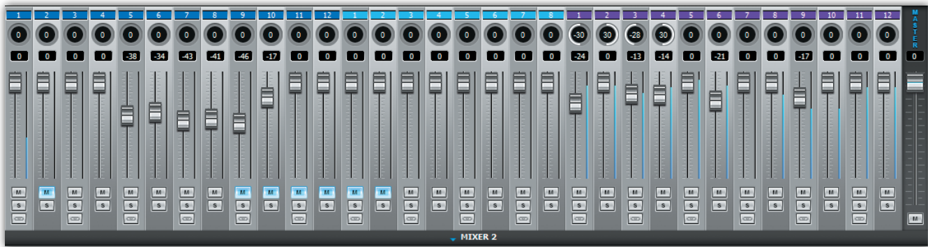
The control panel features four 32-input DSP mixers, each with its own master fader (right).
